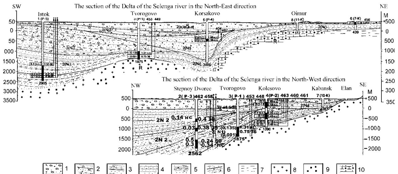
**Figure 2.10.** Hydrogeological cross-sections of Usty-Selenginsk artesian basin. 1: gravel-pebble-sandy sediments, 2: gravel-pebble deposits with sand and interlayers of clay, 3:- intercalation of sand, clay, shale and siltstone and sandstone, 4: gneiss, 5: granites, 6: granite and gneiss, 7: quartzites. Well – top: location; figures from the bottom: depth (m); black-out in the well: tested interval (Tulochonov and Plyusnin, 2008)
