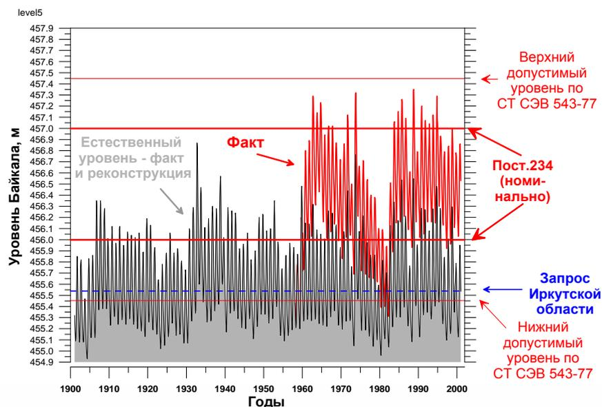
**Figure 4.3.3.a** Fluctuations of the water level in Lake Baikal before and after reconstruction of the dam for the Irkusts hydropower station between 1956-1958. Nominal permissible levels of 456 m and 457 m asl are denoted with bold red lines (RAS 2003).
