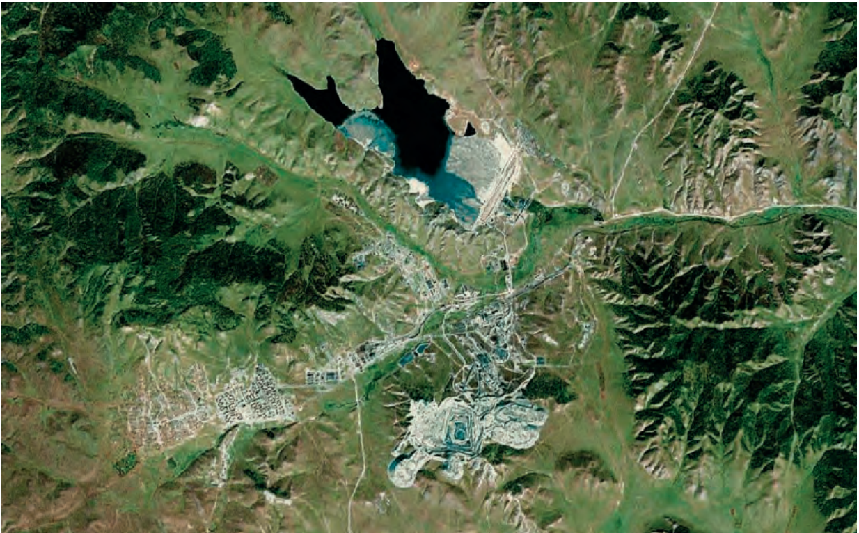
Production and social infrastructure facilities at the copper molybdenum deposit Erdenetiyn Ovoo. There is a tailings pond in the northern part of the photo. The open pit is shown in the southern part, while production and residential zones – in the southwest.
