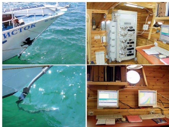
Pic. 5.4.1 The onboard measurement complex «Akvatoria-Baikal»
